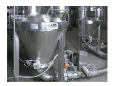
Specifically, when using vacuum conveying, ambient or conditioned air enters the system in a controlled manner. That air (typically from the indoor area of a plant) does not add heat to the product being conveyed. With pressure conveying, a blower is used that forces air into a small space and releases it. In doing this, the air becomes hot and there is a risk that degradation can occur in certain ingredients that are temperature-sensitive.
