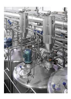
Since the conveying air velocity is much lower in a dense-phase system than a dilute phase system, by comparison, particles are subjected to less degradation or segregation. The material is not moving as fast as dilute and not therefore at risk of breaking.
