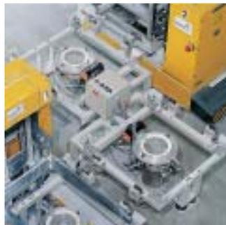
Fully automated, contamination-free product pickup using a pneumatic double door.
