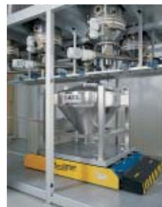
Collecting and weighing of ingredients with the AZO MIXTAINER® and AGV.
