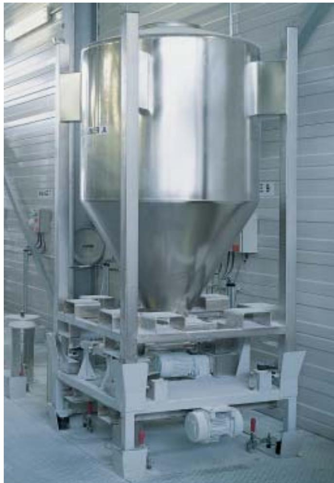
Pickup station with integrated metering screw drive and attached DOSITAINER®.
