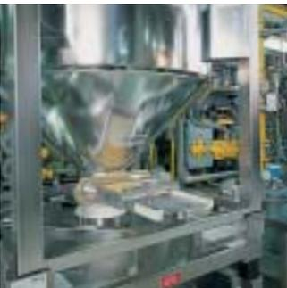
Contamination-free, manual product pickup via a modular gate valve.
