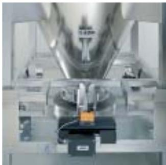
Automated opening of the manual outlet valve using a pneumatic rotary drive.
