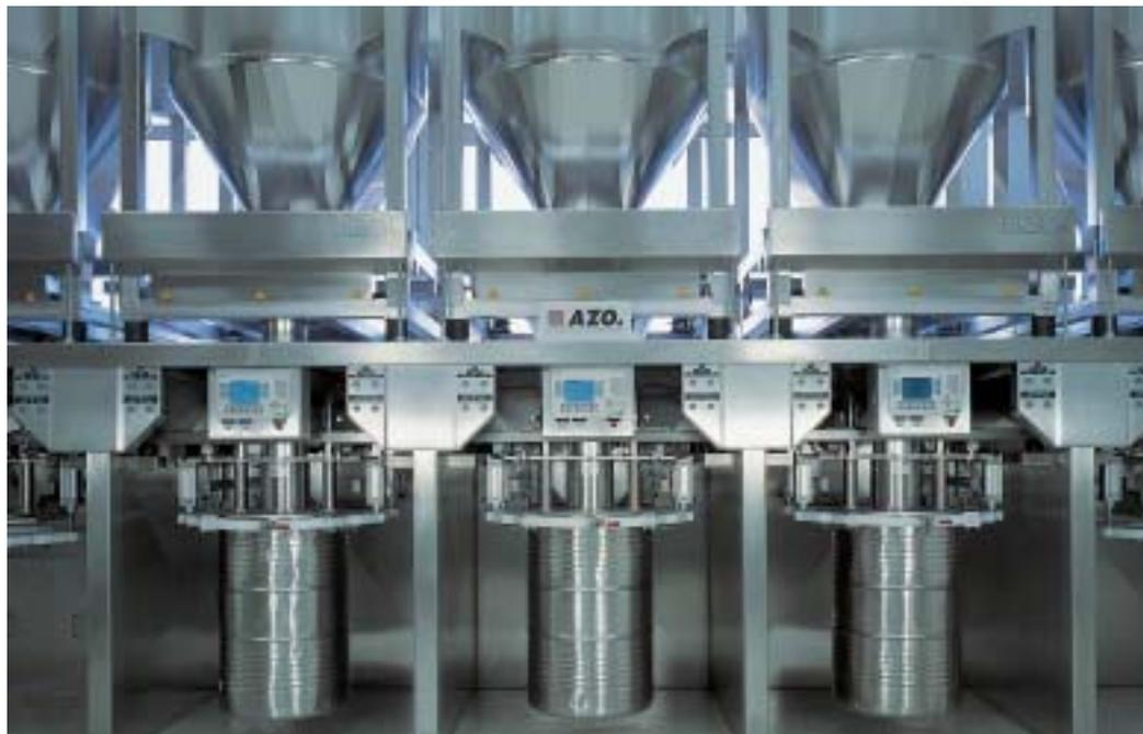
Centralized weighing of active and carrier ingredients into drums via the DOSITAINER®.
