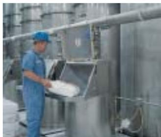
In addition, micro ingredients are manually weighed with the highest precision under operator guidance and then transferred into the container.
